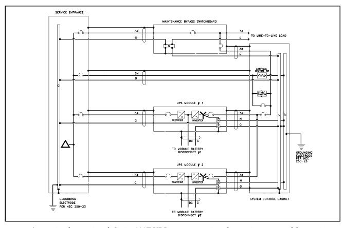
As previously mentioned, Series 600T UPS systems require a bypass input netrual for sensing and monitoring. With a wye-connected input source, the installer should always connect the building service neutral to the System Control Cabinet (SCC) output neutral to achieve this. When the building service is delta-connected, however, the installer must take special steps to ensure reliable UPS functioning.
